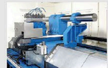
Boring bar toolholder with linear rails
