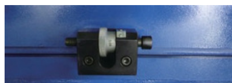
Micrometer Carriage Stop (Positioning system and auto power off)
