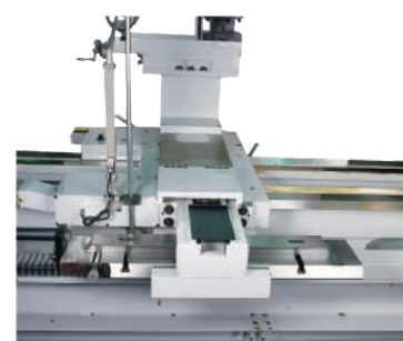
Taper turning attachment ±7 degree Travel:500mm(19.68")
