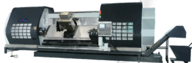
SS/SA/SB series(with Y-axis) Spindle bore 6" Swing over bed 31" Distance between centres 120"
